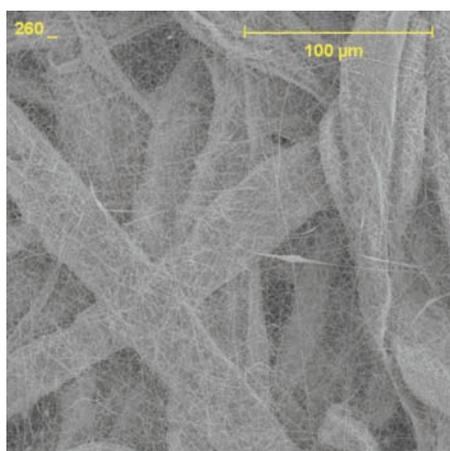
**Figure 3.** Top View of Electrospun Nanofiber Coating, 260X
