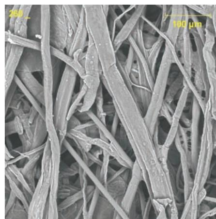
**Figure 2.** Top View of Standard Cellulose Media, 260X
