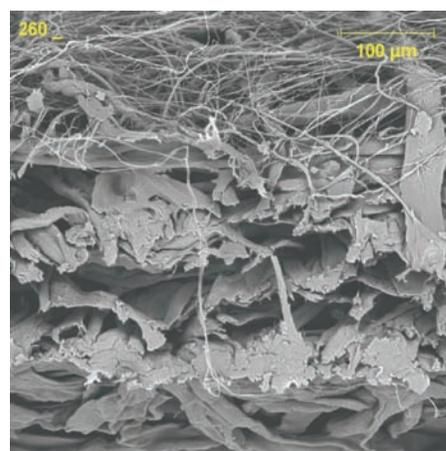
**Figure 4.** Side View of Nanofiber Coating, 260X
