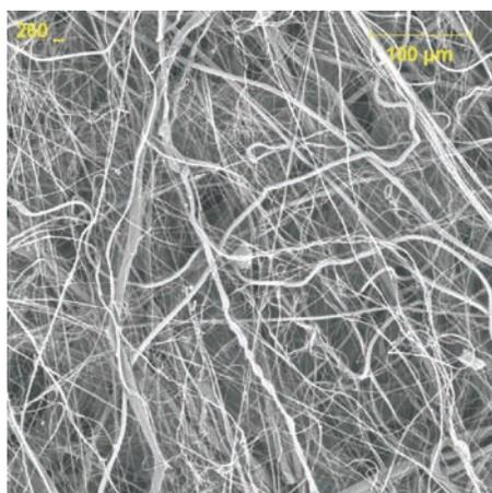
**Figure 1.** Top View of Nanofiber Coating, 260X
