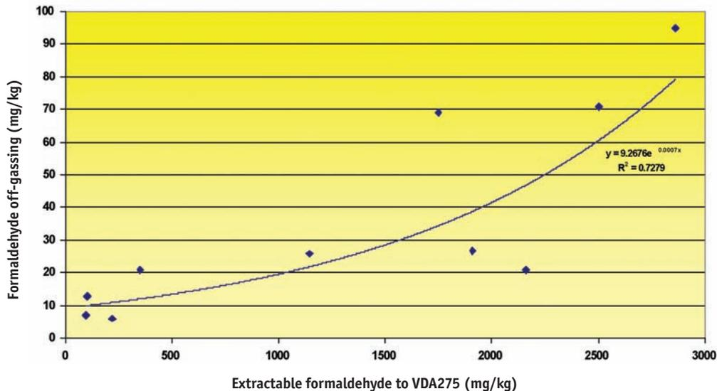
Compared to melamine-based resin technologies, phenolic resins lack ability to generate additional formaldehyde with additional heating. Consequently, testing shows a reduction in emissions with increasing pre-cure for standard cure phenolic media (Figure 5), with a strong exponential decay.
