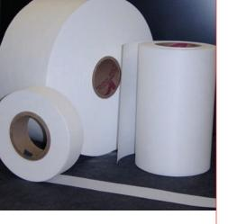
More robust hybrid separators can actually reduce battery assembly costs as compared to 100% microglass AGM types. The force that the separator applies to the positive and negative plates gives a VRLA battery much greater vibration resistance for off-road or heavy-duty equipment. One company reported their VRLA product has twelve times the vibration resistance over conventional flooded batteries.
