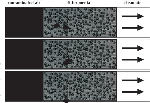
Filtration takes place through a combination of processes: diffusion for 0.3 micron and smaller droplets; inertia and impaction for droplets of 1 to 20 microns. When droplets coalesce to a size of 20+ microns, gravity draws them out of the stream.
