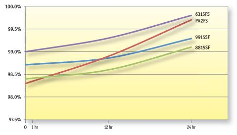
*Examples: Four different H&V nonwovens are subjected to a 10% stretch and hold over 24 hours, with these resulting excellent recovery curves.*
